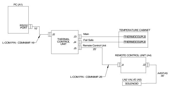
Figure 9 Thermal Control System Cabling
