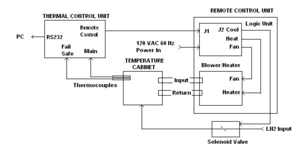
Figure 1 Thermal Control System configuration.
