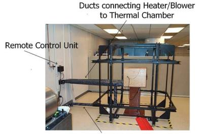
Insulated LN2 line Connection to Thermal chamber
