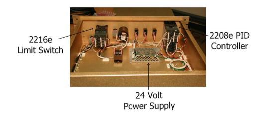
Figure 4 Rear View of Controller Interior
